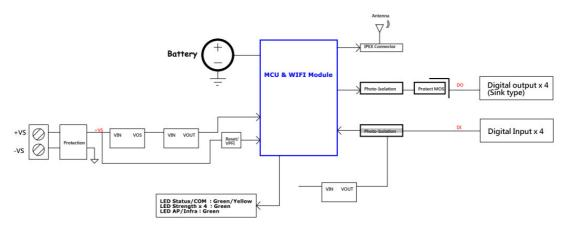
Figure 2.21 WISE-4050 Block Diagram
