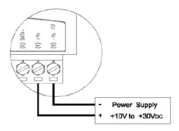
Figure 3.10 Power Supply Wiring
