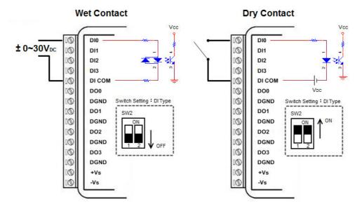
Figure 2.18 WISE-4050 Digital Input Wiring Diagram
