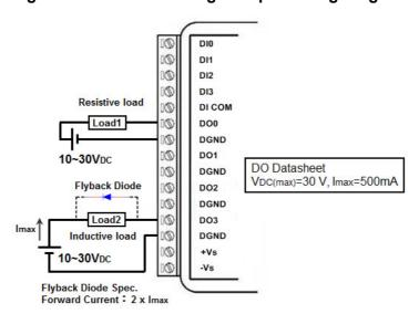
Figure 2.19 WISE-4050 Digital Output Wiring Diagram
