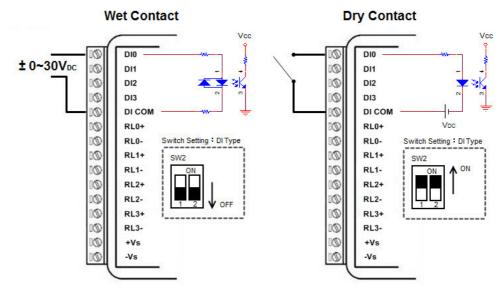
Figure 2.9 WISE-4060/LAN Digital Input Wiring Diagram
