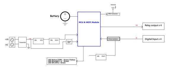
Figure 2.25 WISE-4060 Block Diagram
