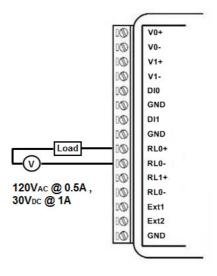
Figure 2.15 WISE-4012E Relay Output Wiring Diagram
