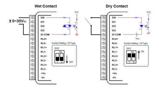
Figure 2.22 WISE-4060 Digital Input Wiring Diagram
