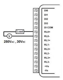
Figure 2.23 WISE-4060 Relay Output Wiring Diagram
