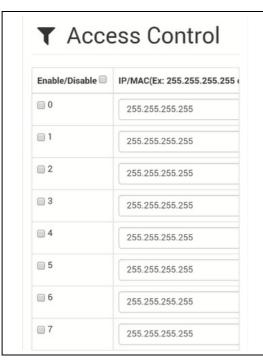
Enable one of the rows and enter the IP address or MAC address which allows to access the WISE-4000 device.
