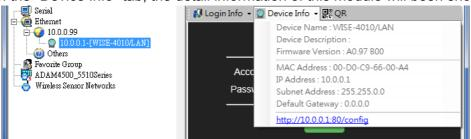
The "QR" tab will generate the QR code of the web configuration web page for mobile device to access the module. User can also click the QR code to open the browser for further configuration.
