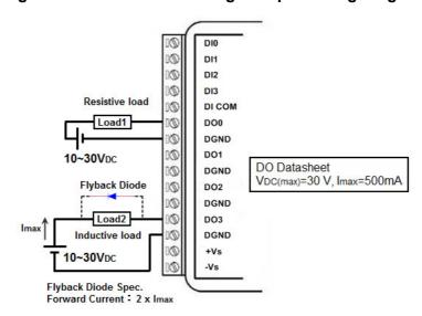
Figure 2.6 WISE-4050/LAN Digital Output Wiring Diagram
