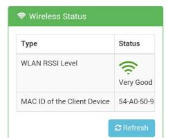
For WISE-4000 Wireless Series, user can check WLAN RSSI Level to know the signal quality in Wireless Status part. And it also shows the MAC ID of the client device.
