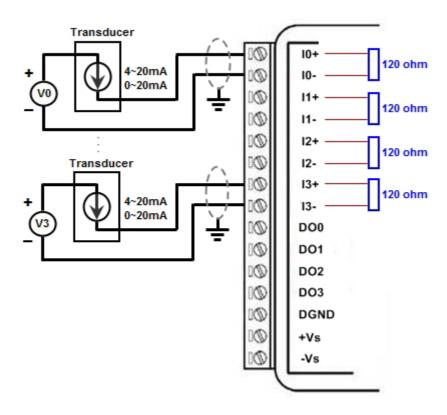
Figure 2.1 WISE-4010/LAN Current Input Wiring Diagram
