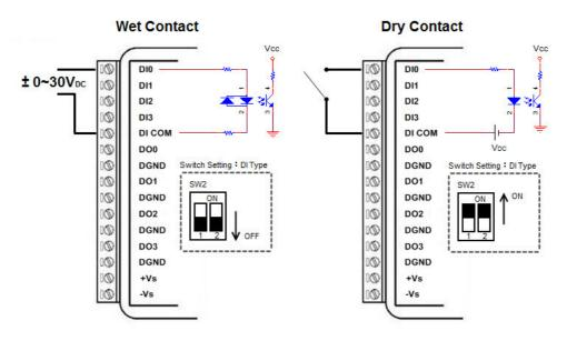
Figure 2.5 WISE-4050/LAN Digital Input Wiring Diagram
